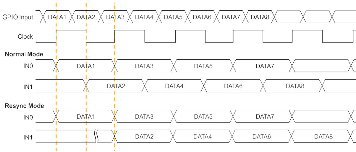
In resync mode, the IN1 data captured on the falling clock edge is delayed one half clock cycle.
