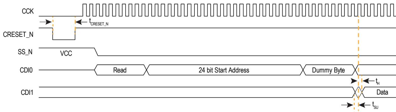
Figure 28: SPI Passive Mode (x1) Timing Sequence
