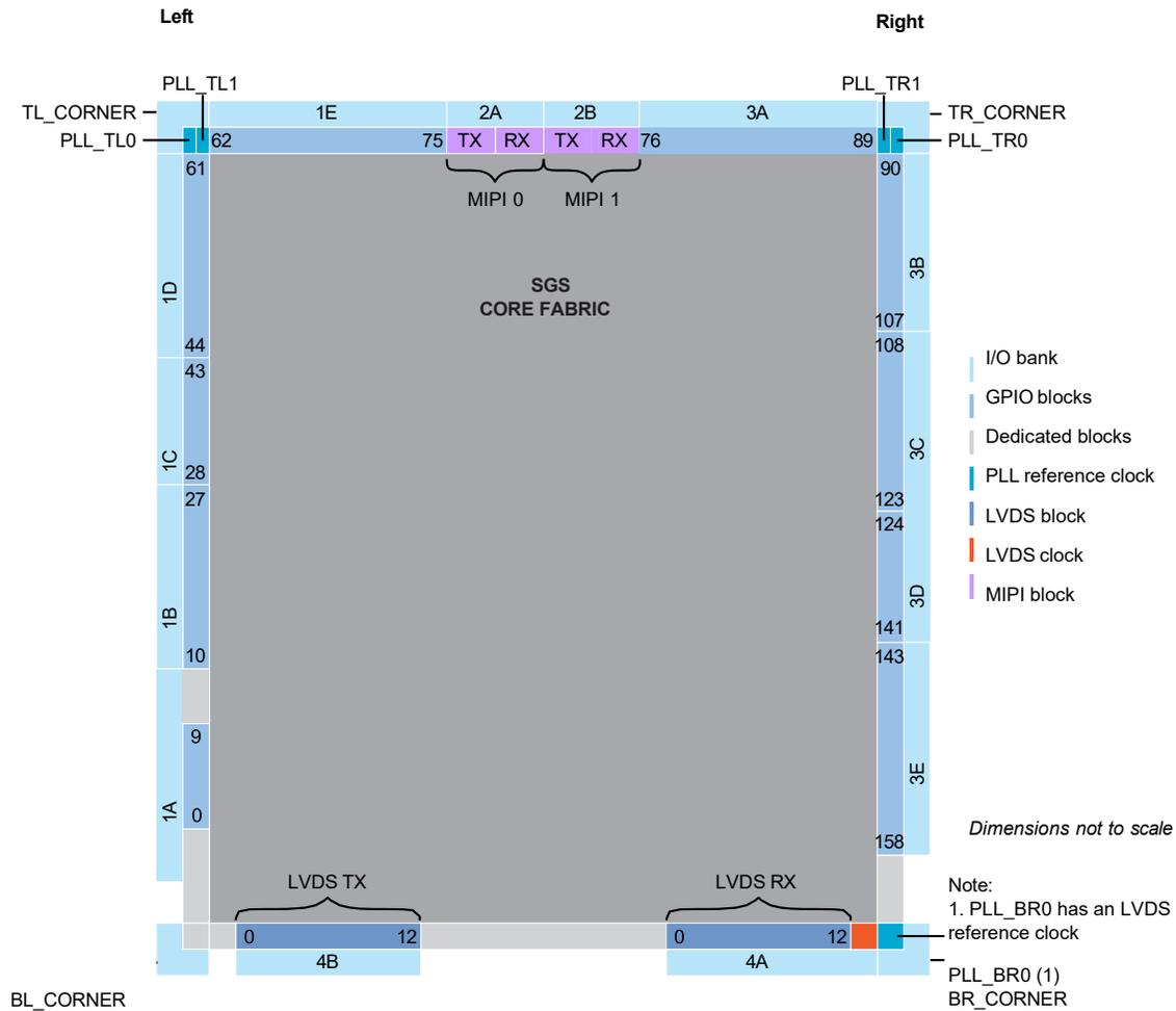
Figure 31: Floorplan Diagram for FPGAs in BGA176 Packages
