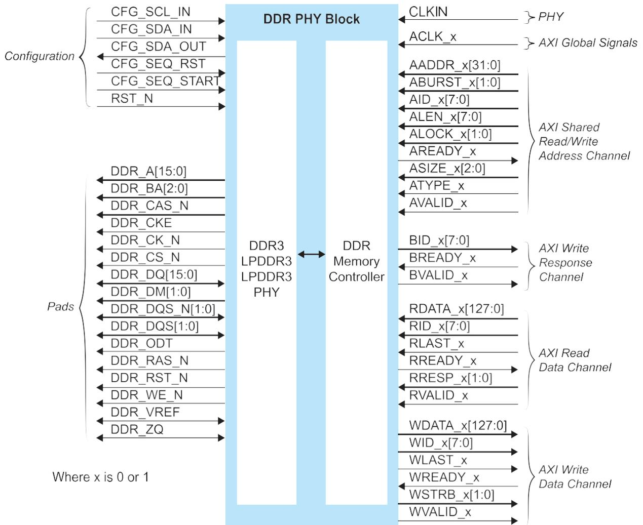
Figure 25: DDR Interface Block Diagram
