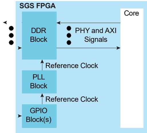
**Note:** Although the PLL reference clock can be driven by I/O pads or the core clock tree, SGS recommends using an I/O pad. The clock tree may induce additional jitter and degrade the DDR performance. Refer to [PLL](#) on page 15 for more information about the PLL block.
