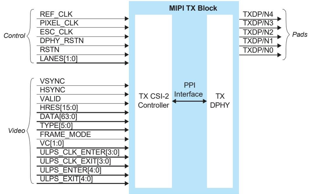
The control signals determine the clocking and how many transceiver lanes are used. All control signals are required except the two reset signals. The reset signals are optional, however, you must use both signals or neither.
